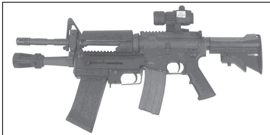
Figure 3-10. M26 Modular Accessory Shotgun System completely mounted to the host weapon
