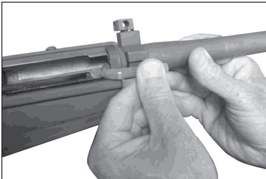
Figure 2-15. Inspecting the bore using a bore reflector
